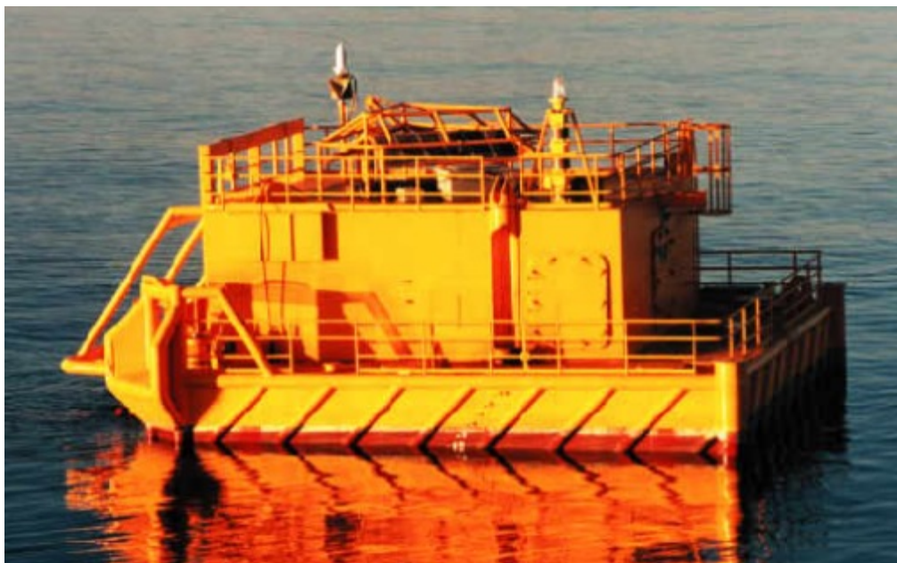
Figure 7 A Catenary Anchor Leg Mooring buoy
