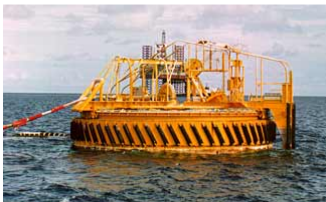
Figure 20 A Single Point Mooring buoy
